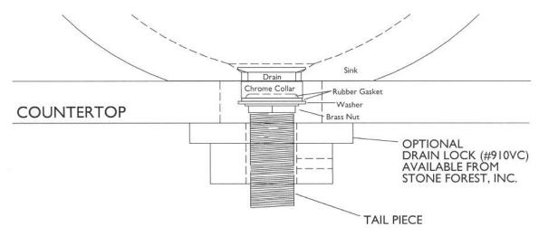
Required drain use 9054D Grid Drain. Drains are 1.25" NPT. This can be supplied by Stone Forest at your request in select finishes.
