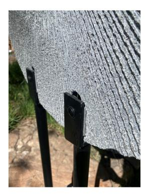
4. The provided barrel bolts should be installed with washers on each side on the outside of the iron prongs as shown below.
