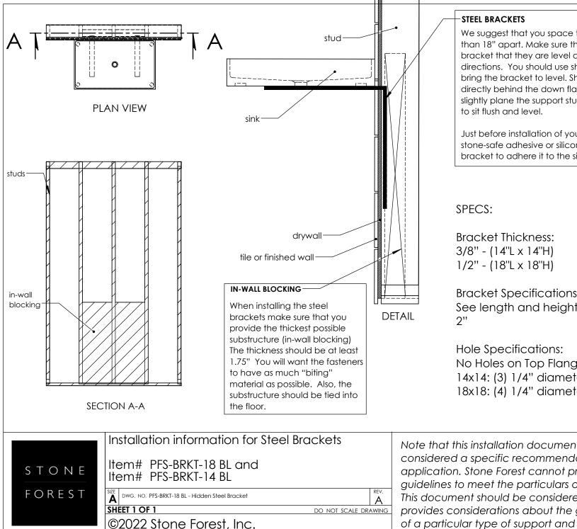
We suggest that you space the brackets no greater than 18" apart. Make sure that when you fasten your bracket that they are level and plumb in all directions. You should use shims in your installation to bring the bracket to level. Shims can be placed directly behind the down flange or you may need to slightly plane the support stud to allow for the bracket
