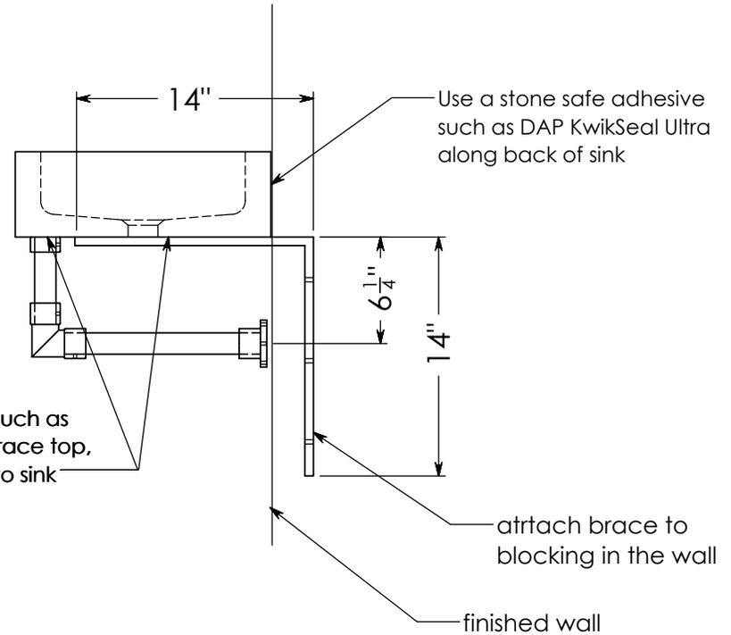
Use a stone safe adhesive such as DAP KwikSeal Ultra along brace top, and where brass attaches to sink
