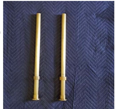
5) Leg assembly using 31" tube, foot and collar.
