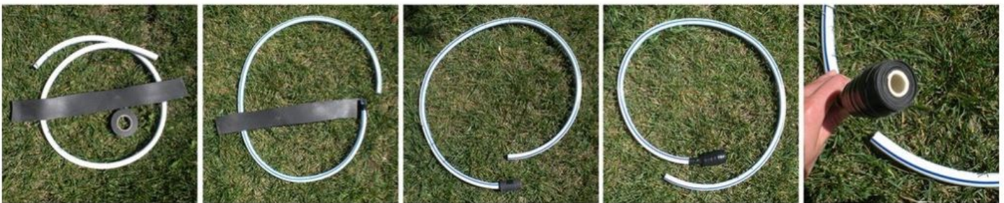
steps to creating the plug end of the hose
